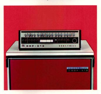
The DDP-516 console is cable-connected to the central computer and can be positioned anywhere on the top of the cabinet to suit operator convenience. Or it can be moved to an adjacent table if preferred.
