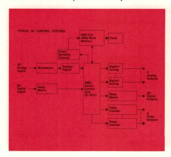
3C, with more than twelve years of digital systems development experience incorporating time tested digital logic modules, has delivered a wide variety of computer systems. These range in design and complexity from multi-loop process control, computerized analysis of speech patterns, to real-time digital flight simulation.
