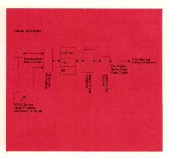
reservation availability. The system employs dual central processors, each time sharing disc and magnetic tape units through programmed electronic switches. Sixteen low and medium speed data communications circuits are switchable between either central processor.
