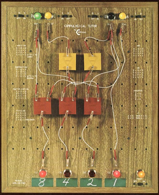
The "output" or the computer's guess as to the number the individual has selected is shown at the bottom of the panel. The output lights have positional weight, according to the 8-4-2-1 code used by today's computers. Light to the right location has a value of 1; the next light to the left has a value of 2; the next
